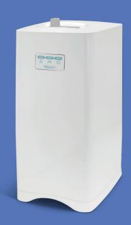
Connect READER directly to your computer and start scanning; three LED lights will indicate the status of the process. Once you insert the plate into the slot, READER automatically recognizes its size and in a few seconds the image appears on the PC.
